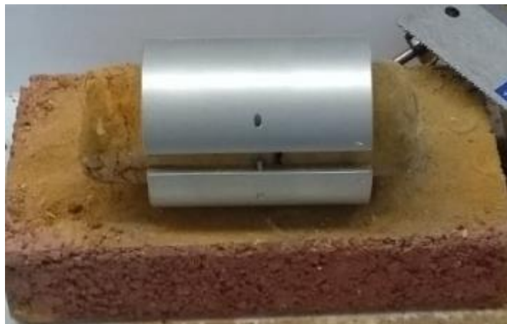
Figure 3.26: Undisturbed sample inside 10 cm split mold.
