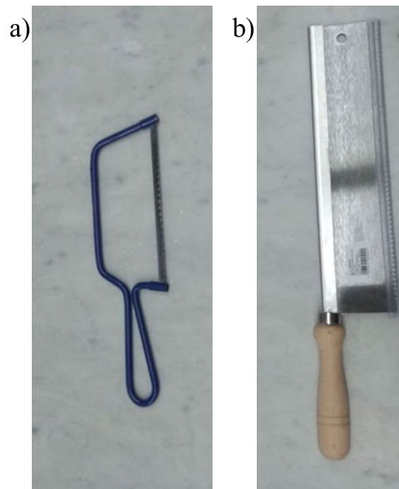
Figure 3.27: Saws used to cut undisturbed samples: a) wire saw, b) wood saw.
