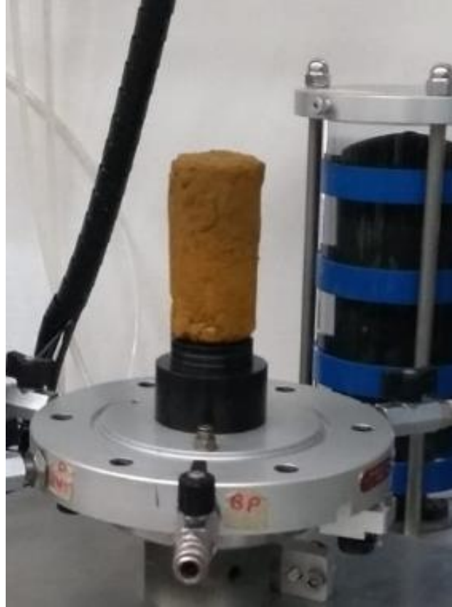
Figure 3.29: Undisturbed sample on the base capital.
