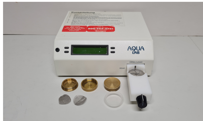
Figure 4.6.: Chilled mirror hygrometer AquaLab CX-3TE used in this study with a plastic lid for loose samples and a closed and an open microcell with meshes for samples at constant volume conditions.
