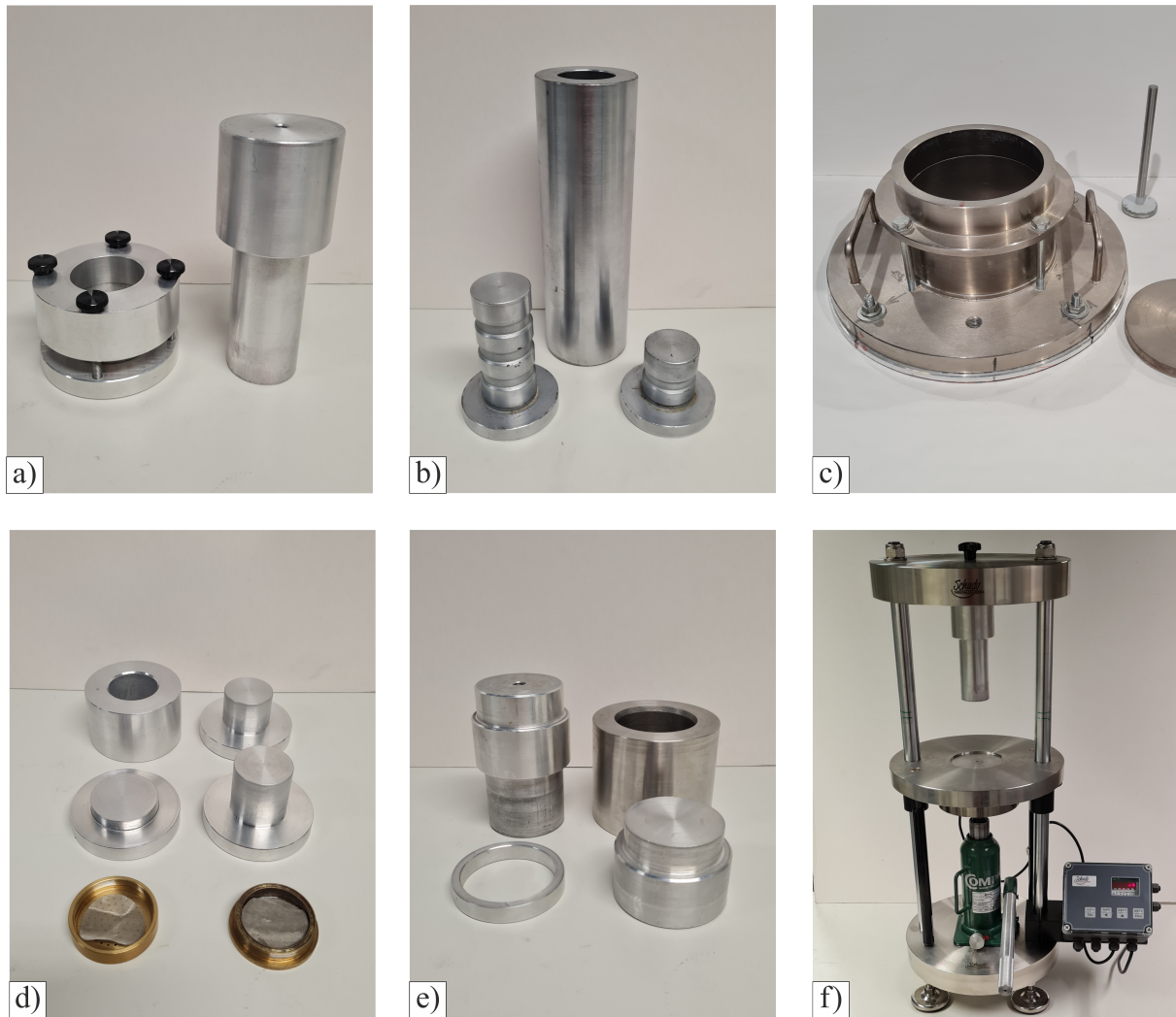
Figure 4.4.: Compaction sets used in this study for compacting samples for: a) swelling pressure and oedometer tests directly into the sample ring, b) triaxial and thermal conductivity testing, c) the investigation of compaction induced anisotropy, d) SWCCs with direct transfer into microcells and e) swelling pressure tests in the newly developed cell for tunnelling relevant boundary conditions directly into the sample ring. f) Shows the used hydraulic jack for densities up to 2.0 \text{ g/cm}^3 with an integrated load cell.
