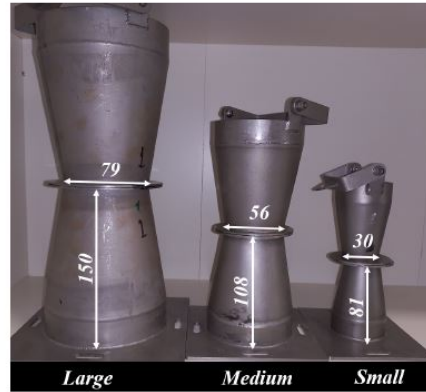
FIGURE 4.10 – Three differently sized conical devices for tensile traction tests (FARHAT 2023)
