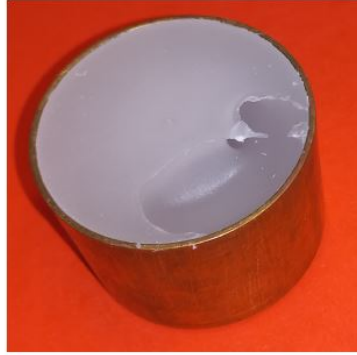
FIGURE 4.7 – Commercial paraffin used as binder between particles (FARHAT 2023)
