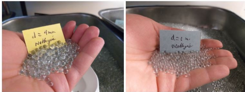
FIGURE 4.6 – Spherical glass beads with diameters 3 mm and 4 mm (FARHAT 2020)
