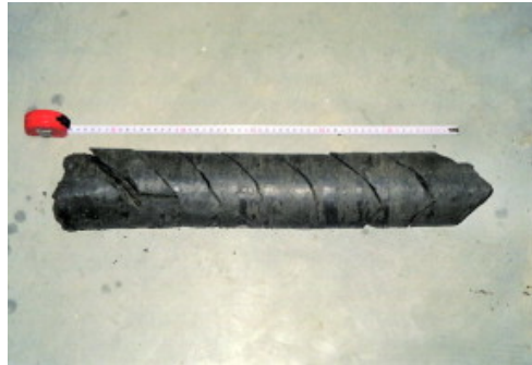
Figure 2.22.: Fractures pattern along a Boom Clay borehole core induced by the drilling process (Wileveau and Bernier, 2008)
