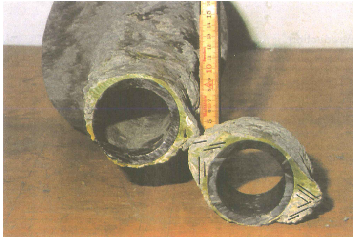
Figure 2.23.: Eye shaped combined shear-extensional fractures around a borehole in OPA (Thury and Bossart, 1999)
